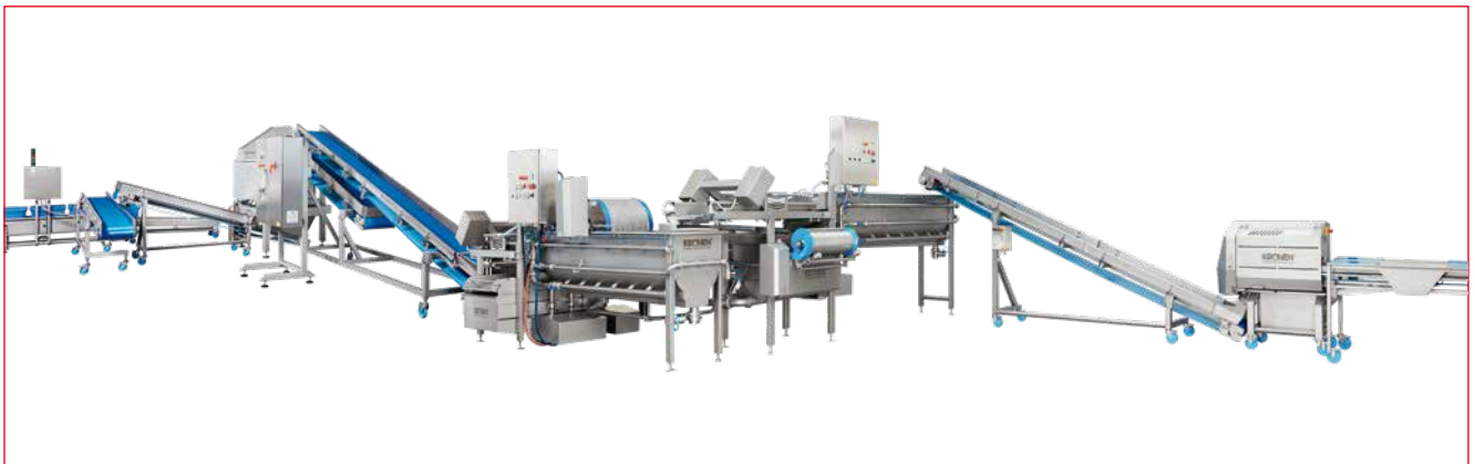
Sweden: Processing line for cutting, washing, drying and weighing lettuce and different vegetables - capacity up to 1000 kg/h
