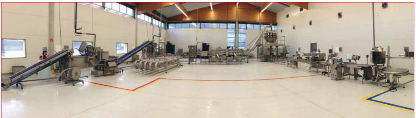
Austria: Processing line for trimming, slicing, washing, treating, spin-drying and mixing leaf salad - capacity up to 500 kg/h.
