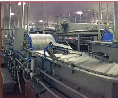
United Kingdom: Large salad processing line – capacity up to 1.500 kg/h Iceberg lettuce and up to 800 kg/ Baby leaf.
