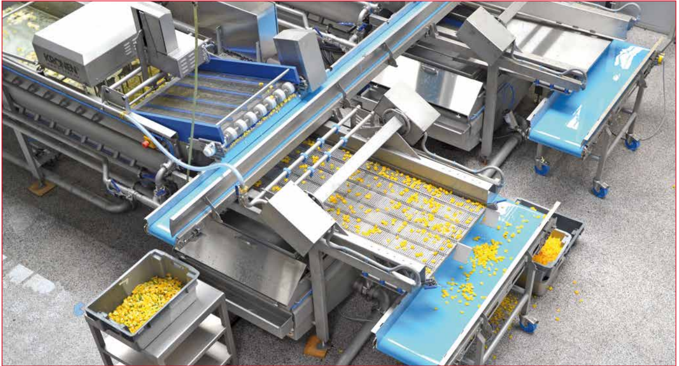
Portugal: Processing line for washing & sorting bell peppers - capacity up to 7 tons/h.
