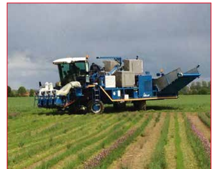
Germany: Harvest & slice cut at chives field with 4 big KRONEN GS 20 belt cutting machines – capacity up to 1,8 tons/h
